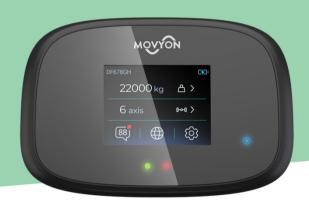
OBU GO Sat is an On Board Unit (OBU) for toll payment using both satellite technology, by sending geolocation data to the central platform via 4G LTE Cellular Network, and DSRC technology. Vehicle localization and route monitoring also allow it to be used for emergency fleet management and for heavy vehicle and urban public transportation tracking.
